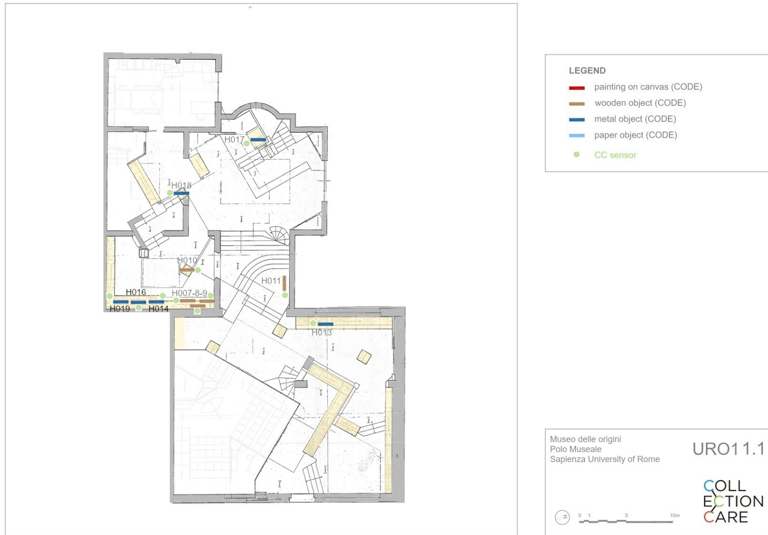
Figure 14. Museo delle Origini: Identification of the eleven sampling points in the plan where fixed sensor node devices (CC sensor, green dots) can be deployed according to the artwork-related deployment . Objects are coloured in accordance with the main material typology as reported in the legend, whereas showcases are marked in yellow. The plan was derived from the original document provided by Dr Cecilia Conati
