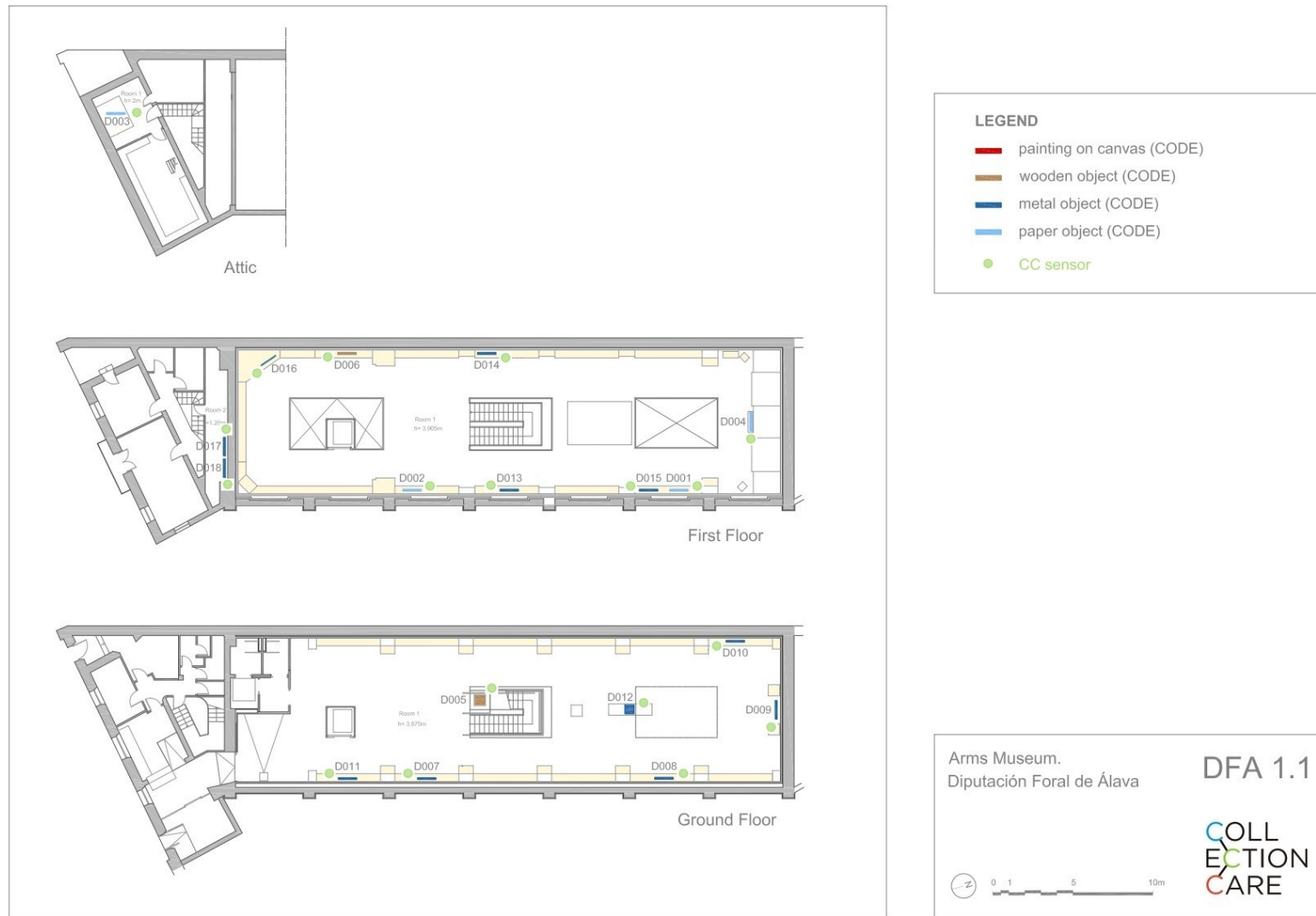
Figure 11. Alava Arms Museum (AAM): Identification of the eighteen sampling points in the plan where fixed sensor node devices (CC sensor, green dots) can be deployed according to the artwork-related deployment . Objects are coloured in accordance with the main material typology as reported in the legend, whereas showcases are marked in yellow. The alphanumeric code of the sensor is not displayed for better readability
