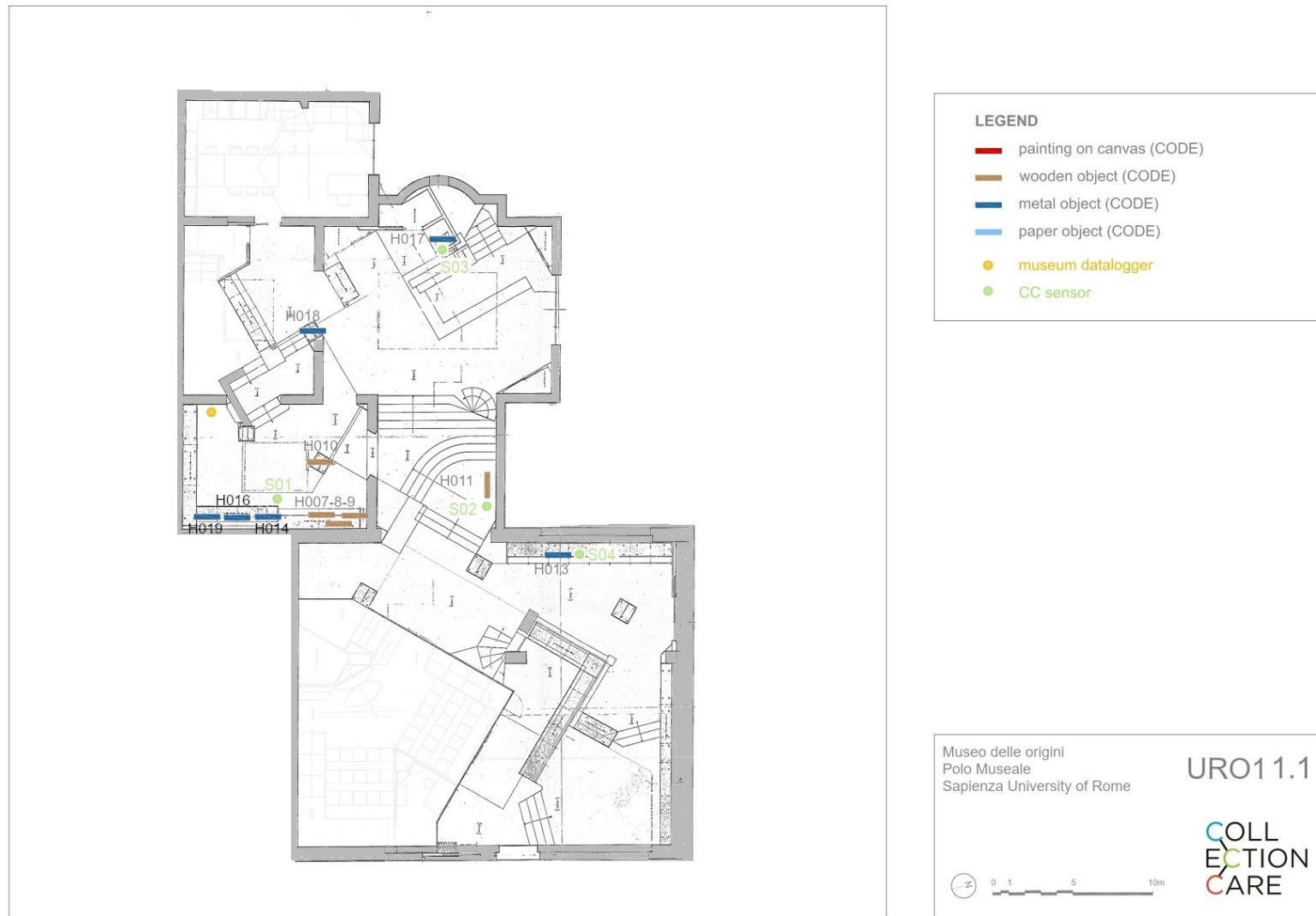
Figure 25. Museo delle Origini: Identification of the sampling points in plan where fixed sensor node devices (green dots) can be deployed according to the artwork-envelope-related deployment associated with Museum Scenario II
