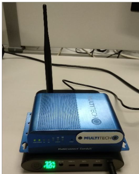
Figure 13. Multitech's Conduit AEP modified LoRaWAN gateway used to test the proposal
