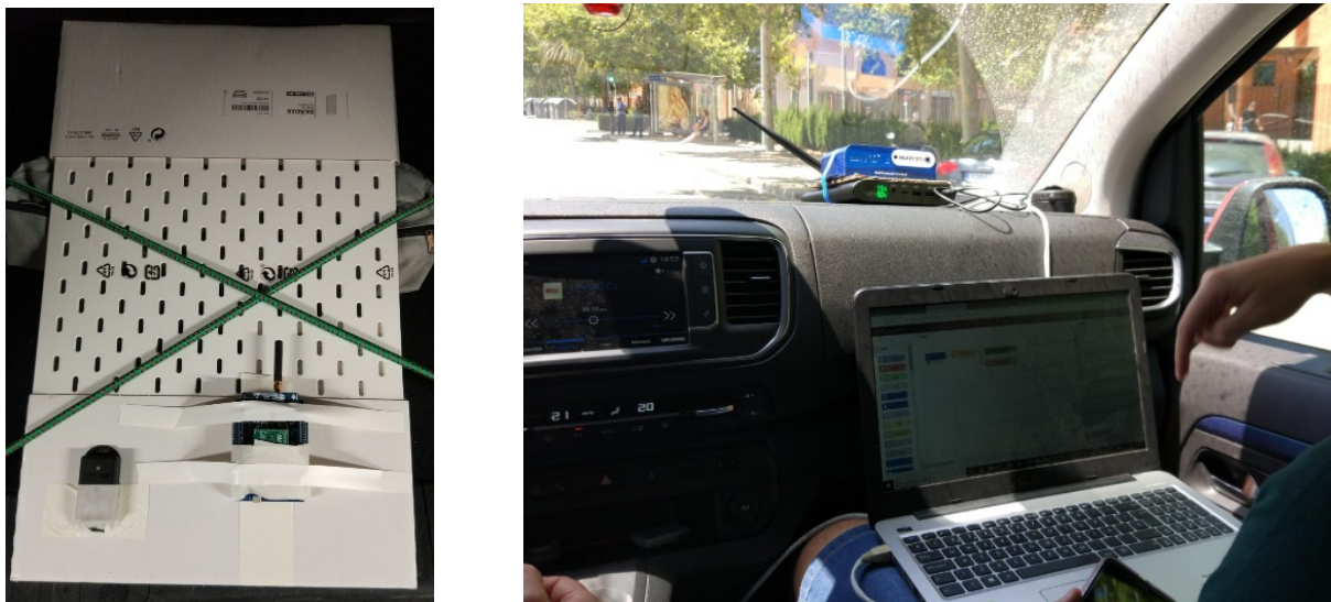
Figure 15. (left) Test piece with datalogger and sensor node attached and boarded in a van. (right) Gateway and laptop installed in the driver's cabin to receive sensor data
