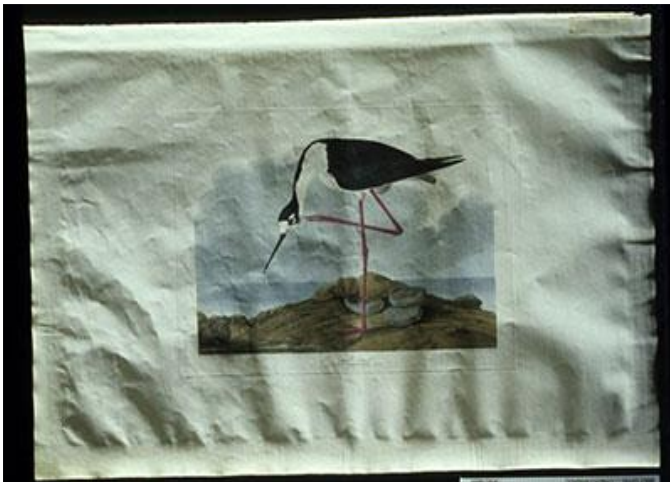
Figure 1: Cockling of an intaglio print, due to moisture fluctuations. Canadian Conservation Institute (Source: www.canada.ca/en/conservation-institute )
